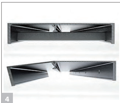
4 Chamfered side and end rails facilitate stripping from the completed structure
