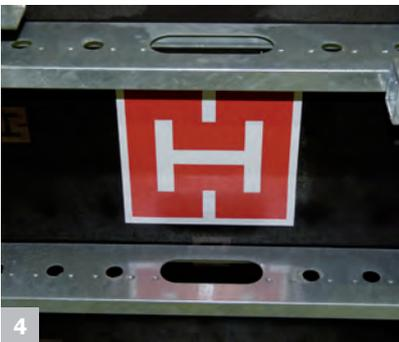
4 Swift handling as well as an ergonomic manual transfer due to integrated grip holes
