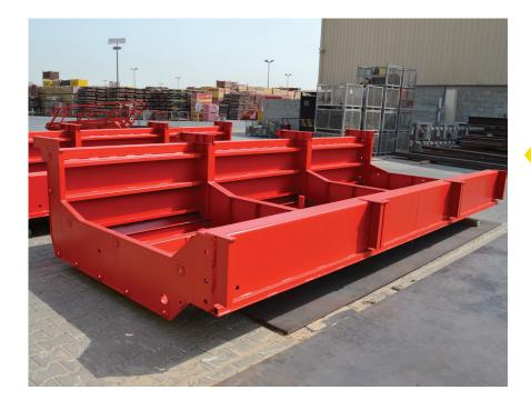
Section for cast in-situ, pier head formwork, with multiple re-uses.
